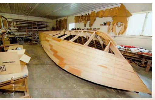
Each Streblow is built by hand, with skill and precision, starting with the keel and ribs, which are then framed with white oak.
